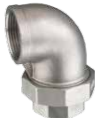
EF9034C Elbow union conic sealing female thread/female thread Material: Stainless steel 316 Size: 1/4"-2"
